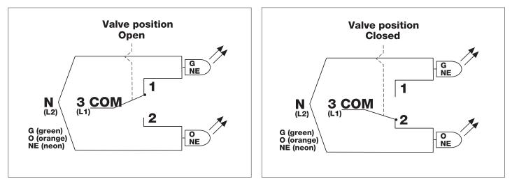
Visual Indicator Indicates closed and open position of the safety valve.
